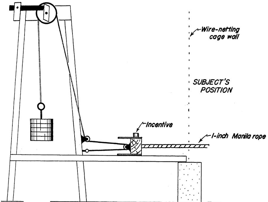
FIG. 1. Diagram of strength-measuring apparatus
